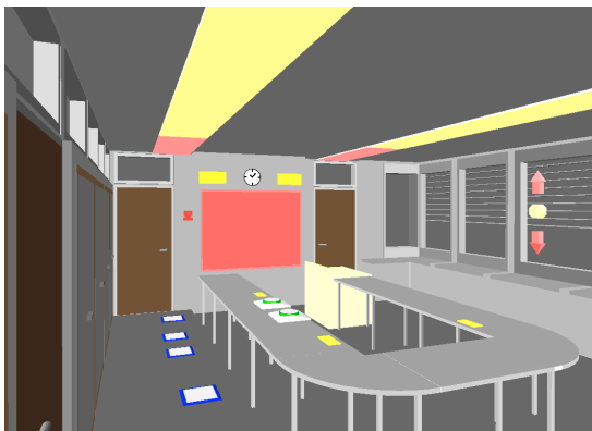
Figure 3. Three-dimensional simulation of our smart meeting room with different virtual installations of pressure plates on the floor and some virtual buttons on the tables.
